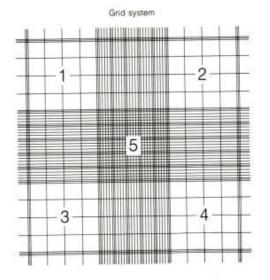
**Figure 3:** The hemocytometer and its grid lines used to determine the total number of cells in a cell suspension.
