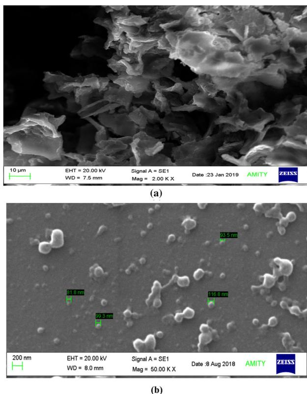
Fig. 3 SEM images of **a** bulk extract of Punicalagin (PCB) and **b** synthesized nanoparticles of Punicalagin (PCN)
